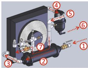
Cooling compressed air and extracting moisture does 50% of the job, an effective efficient dryer must also reheat the compressed air to further separate the air temperature where moisture will occur!
