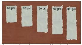
The image above shows an area blasted with different nozzle pressures. Each section was blasted for 5 minutes. This demonstrates how important it is to maintain correct nozzle pressure in order to increase production and decrease abrasive waste. Blasting at 60 psig for 5 minutes cleaned 5 ft² whereas blasting at 100 psig for 5 minutes cleaned 10 ft². "Twice the area in the same amount of blast time."
